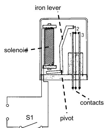
5. This relay has three contacts (see picture). One or two light bulbs can be turned on or off connecting them to the relay in different ways. Pay attention to the fact that an extra voltage source is needed for the lamps - the one in the drawing is used to turn the current for the solenoid on and off
