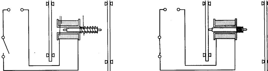
4. A relay is a switch which opens and closes contacts using an electromagnet. This allows for more options than what a simple ordinary switch can do.
