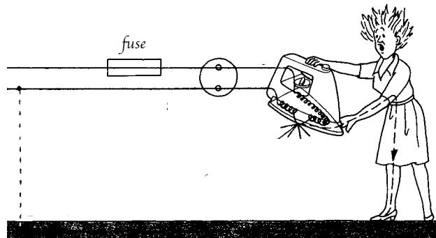
5. Here's a grounded iron with a fuse. Due to a defect in the insulation the outside metal case gets in contact with a current-carrying wire on the inside.
