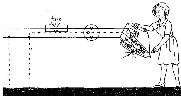
6. Here's an electric circuit protected by a ground fault circuit interrupter (FI circuit breaker).
