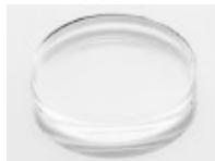
A diverging lens is a flat round piece of transparent material (usually glass), which is thinner in the middle than at the rim. The light rays passing through a diverging lens are bent outward, that is, they diverge.
