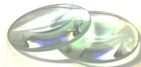
A converging lens is a flat round piece of transparent material (usually glass), which is thicker in the middle than at the rim. The light rays passing through a converging lens are bent inward, that is, they converge.
