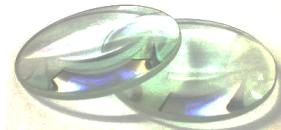
A converging lens is a flat round piece of transparent material (usually glass), which is thicker at the middle than at the rim. The light rays passing through a converging lens are bent inward, that is, they converge.
