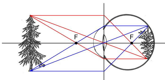
b)  $f = 16 \text{ mm}$ ,  $d_o = 41 \text{ mm}$ ,  $d_i = 26 \text{ mm}$
