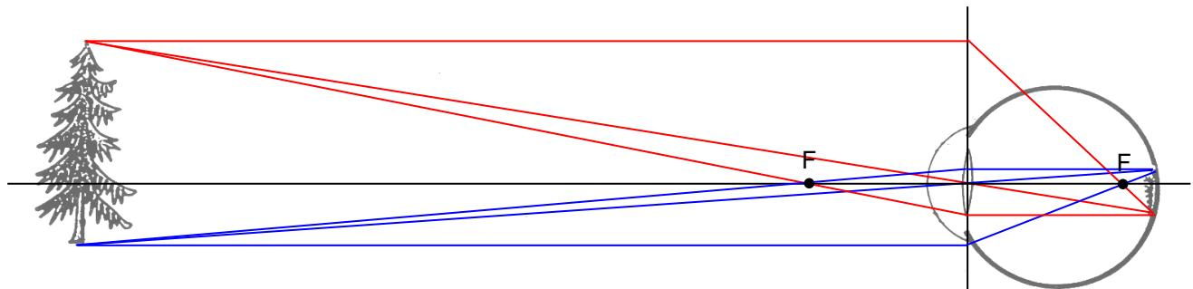
b)  $f = 23 \text{ mm}$ ,  $d_o = 130 \text{ mm}$ ,  $d_i = 28 \text{ mm}$
